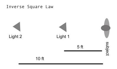
As light travels over distances it spreads or diffuses and in the process it loses intensity (brightness). How much intensity it loses is actually very easy to calculate. We do this by applying a simple formula known as the **Inverse Square Law**. Here is the formula:
